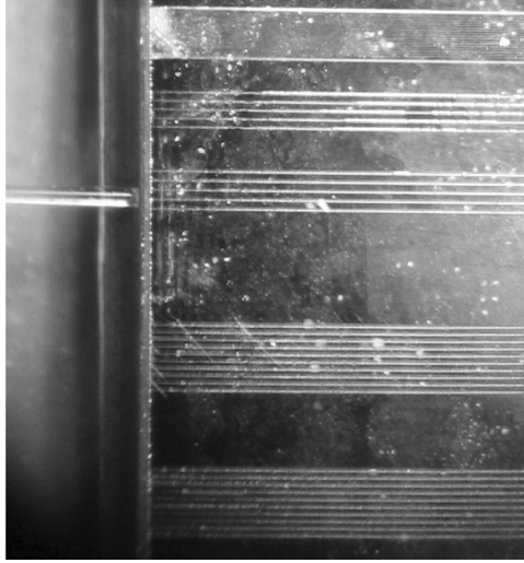
FIGURE 2 Snapshot of LC optical waveguides coupled with a fiber.
